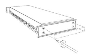
3. From the rear of the cabinet, slide the KVM console onto the mounting rails.
